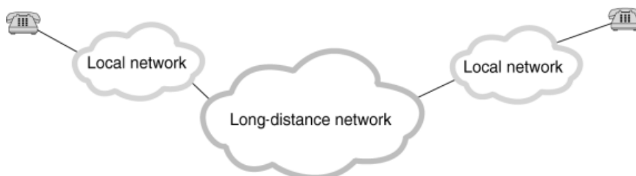
Figure 8.1 General structure of a PSTN.
